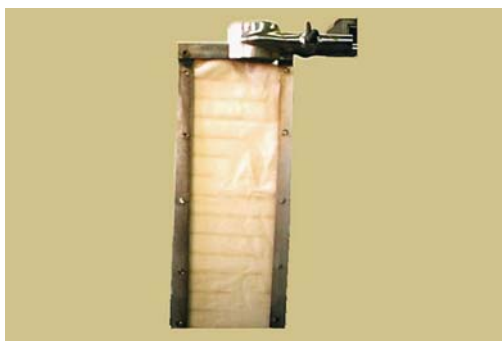
Fig. 1 Mostashari's flammability tester with a treated fabric inserted and pinned in its inner grooves, before to the fulfillment of the flammability test
